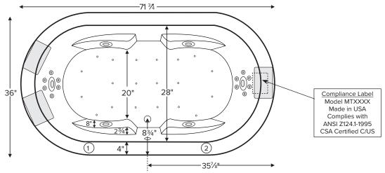
Numbered locations on tub deck represent possible stub-out locations for cleaning systems and valves. If location 2 is chosen for Fill-Flush, the detergent feeder will need to be offset to the left or the right. Shown with Air Massage and Ultra Whirlpool Package.
