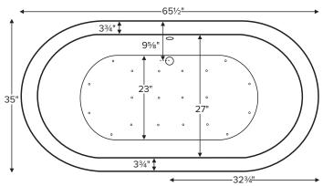
Drain Rough-In Measurements
