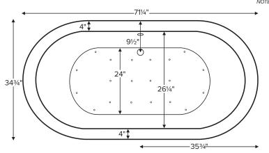
Drain Rough-In Measurements
