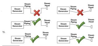
**A WARNING** Failure to pitch the steam piping as required for condensate to drain, may cause condensate to block the flow of steam. Blocking the steam flow may cause steam pressure to discharge boiling water through the steamhead, resulting in a scalding hazard. Blocking the flow of steam may cause steam to discharge through the safety valve, resulting in a scalding hazard.
