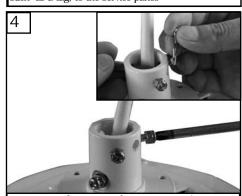
Remove keeper from pin. (see inset) Loosen the 2 set screws in yoke for downrod to slip into yoke.
