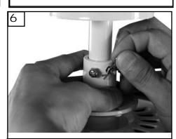
Insert downrod into motor yoke. Next, insert clevis pin through yoke and downrod and secure with cotter pin.
