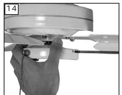
Remove 3 screws from the switch housing plate and save to re-install into the switch housing.
