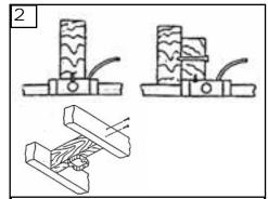
Before installing this fan make sure the outlet box is properly installed to the house structure. To reduce the risk of fire, electric shock, or personal injury, mount to outlet box or supporting system acceptable for fan support. (Mounting must support at least 35 lbs.)
