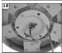
Loosen 2 screws and remove 1 screw from motor plate. Save removed screw for use later.
