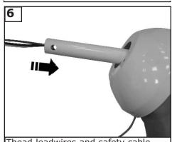
Thead leadwires and safety cable through downrod. (as shown)
