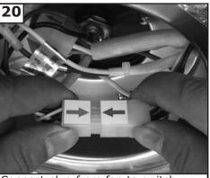
Connect plug from fan to switch house plug.
