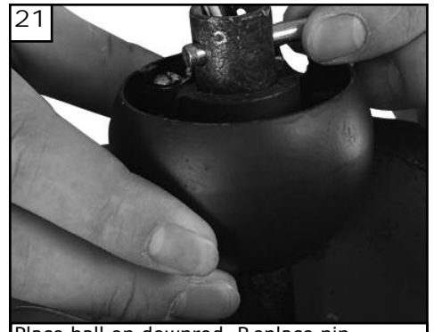
21 Place ball on downrod. Replace pin removed earlier and pull ball up so that the pin fits in the notches in the ball.
