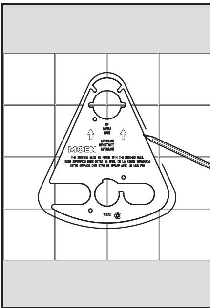
The plaster ground face indicates the correct orientation for the valve assembly, as shown (arrows pointing upward). **CAUTION:** For CC (copper to copper) installations, the cartridge must be removed from the valve body before heating the valve. Failure to do so will result in cartridge damage. Please refer to the instructions 'Cartridge Removal.'
