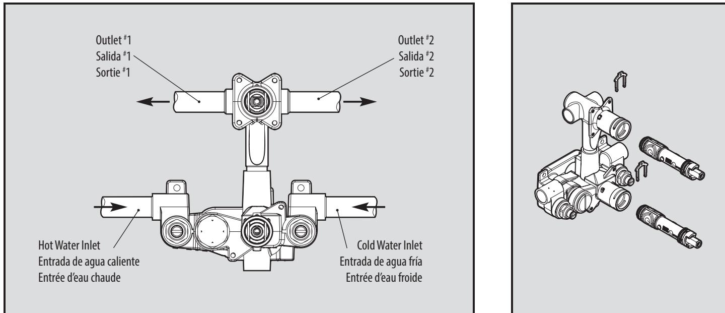
Connect the piping to the valve as shown above. If soldering copper to copper, be sure to remove the cartridges prior to soldering (see Cartridge removal step). **NOTE:** Do not use outlet port on Moentrol Valve. Unplugging and use of this port will cause improper functioning of the valve.
