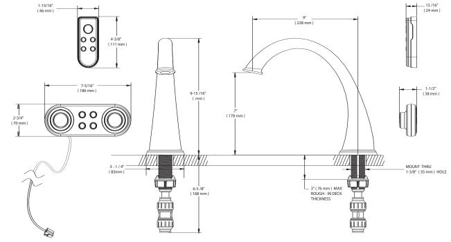
NOTE: THE INSTALLATION SHOWN IS FOR TILE DECKS, THIS VALVE WILL ALSO FIT STEEL, CAST IRON OR PLASTIC DECKS
