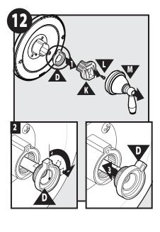
Remove the Lever (M) and Lever Handle Adapter (K). Note the position on the stop. Position the Adjustable Temperature Limit Stop (D) so the Lever stops at the position. This prevents the Lever from being turned into an unsafe temperature.
