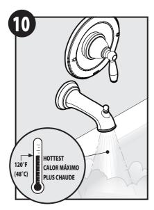
Turn handle on to test hot water temperature. Turn off handle if desired water temperature has been met. Hot water temperature should not exceed 120°F.
