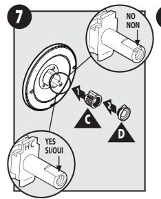
Make sure cartridge stem is positioned with notch facing down. Insert Key Stop **(C)** & Adjustable Limit Stop **(D)** into Stop Tube.
