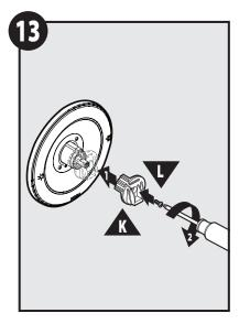
After setting the adjustable temperature limit stop to the desired position, reattach the Lever Handle Adapter (**K**), Adapter Screw (**L**), and Lever (**M**). Make sure ridges on back of (**K**) are to the left of the tab on (**D**).
