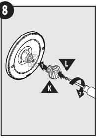
Install Handle Adapter **(K)** onto cartridge stem with Handle Adapter Screw **(L**.
