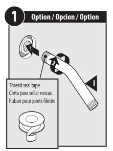
Wrap thread seal tape around Shower Arm (I) threads. Screw Shower Arm into connection in wall.
