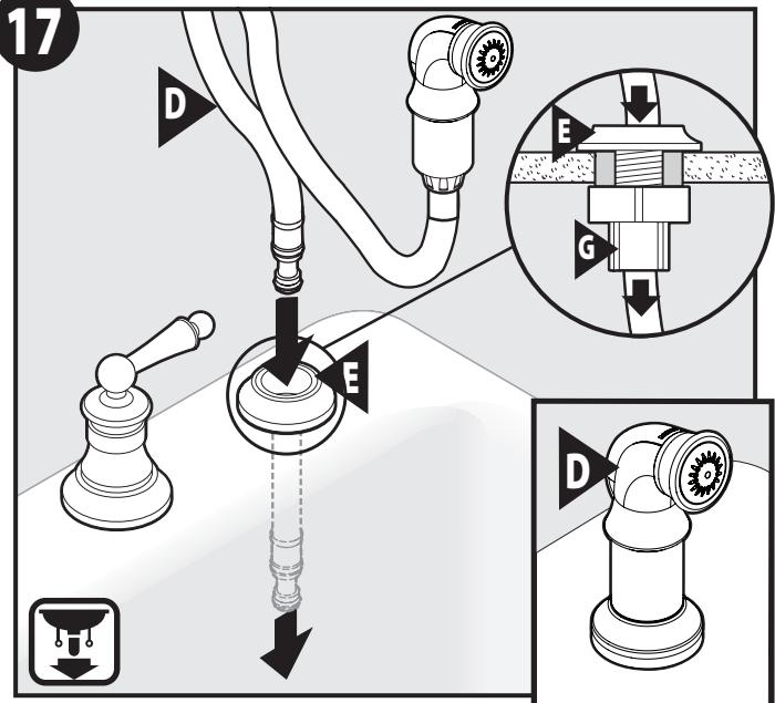
Insert Side Spray (D) through Hose Guide (E) until Side Spray is fully seated.
