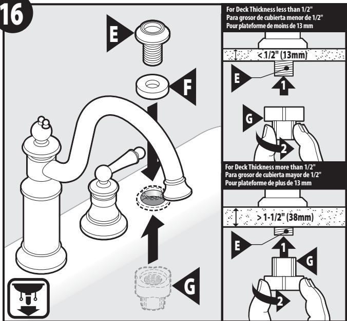
Install Hose Guide (E) and Hose Guide Gasket (F) together into sink opening. Secure with Hose Guide Nut (G). Hand tighten. **Note:** For deck thickness greater than 1-1/2", invert Hose Guide Nut (G).
