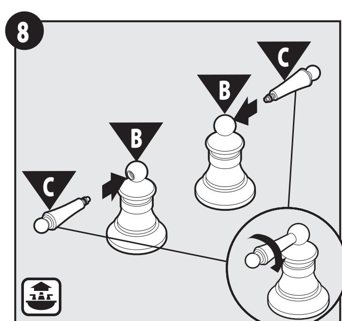
Install Handles (C) to both Handle Hubs (B). Thread by hand until secure. Note: If using optional Temperature Indicator Rings (red and blue), ensure handle with red ring is on the left and handle with blue ring is on the right.
