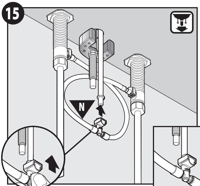
Install center quick connection of Hose (N) to longer shank as shown. Push in as far as possible until a "click" is heard. Tug downward to test engagement.
