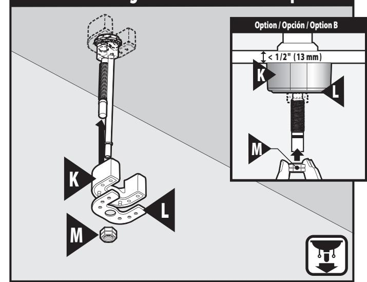
For sinks thinner than 1/2", use the plastic Mounting Bracket (K) and metal Mounting Plate (L). Secure bracket, plate, and spacer with Spout Mounting Nut (M). Thread Nut by hand until secure.
