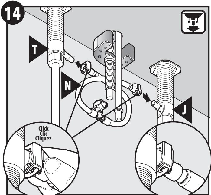
Install each end of Quick Connect Hose (N) to both Valve Bodies (T) and (J). Push in each end far as possible until a "click" is heard. Tug on each connection to test engagement.
