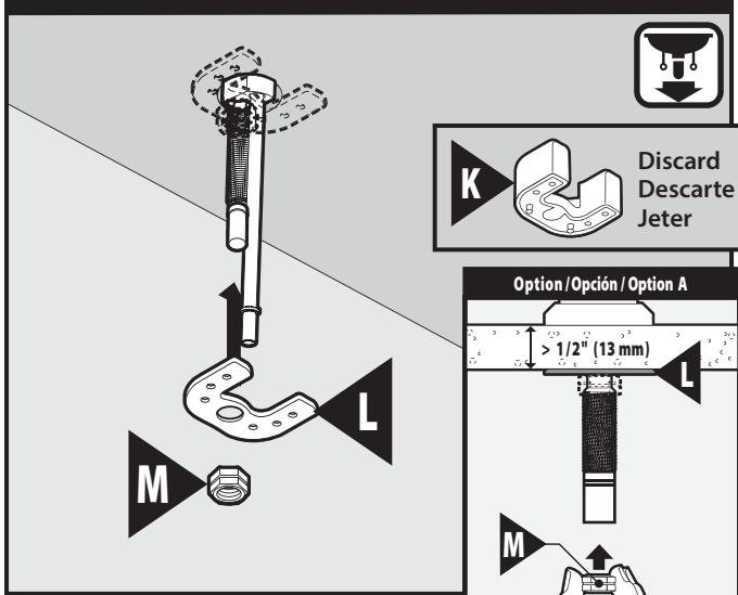
For sinks thicker than 1/2", use the metal Mounting Plate (L) only. Secure plate with Mounting Nut (M). Thread Nut by hand until secure.
