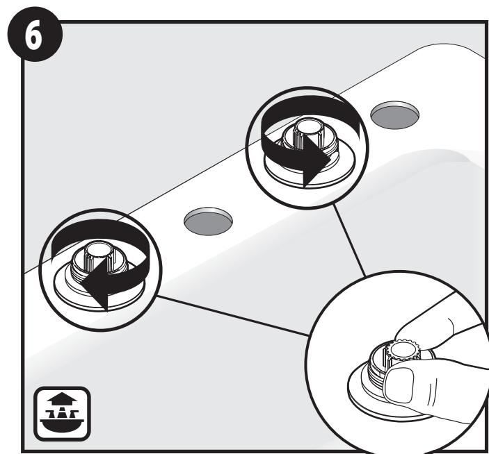
Ensure each valve body cartridge stem is turned to the off position.
