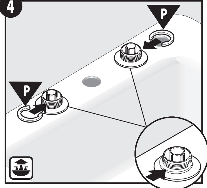
While holding a Valve Body, insert Valve Body Clip (**P**) into groove of each Valve Body. Ensure Clip is within groove.
