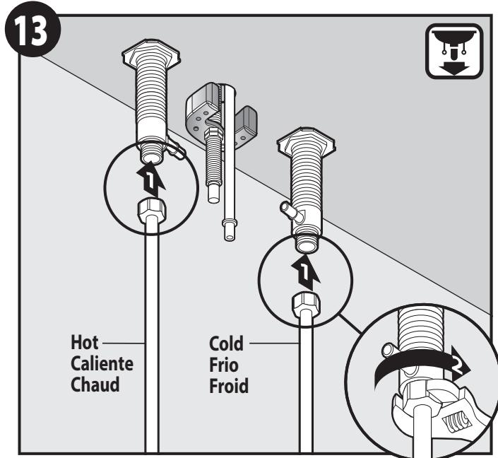
1. Attach hot and cold supply lines (not included) to Valve Bodies.
