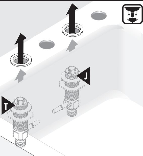
Install both Valve Bodies, Hot (**T**) and Cold (**J**), up through sink openings.
