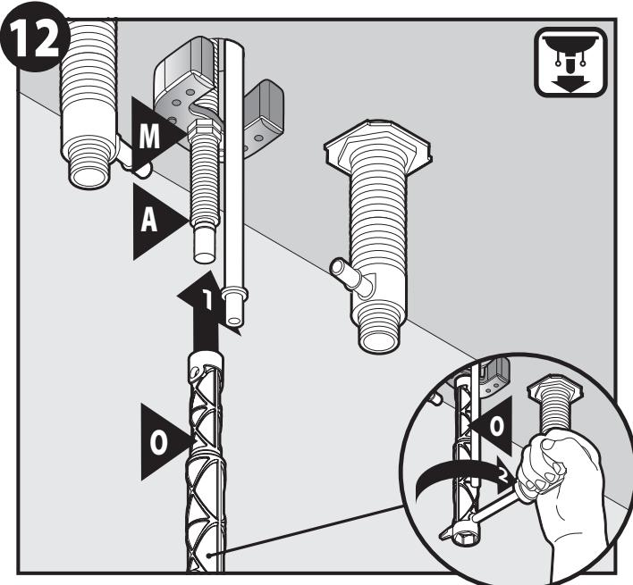
1. Slide installation Tool (O) over shank of Faucet body (A) and onto Spout Mounting Nut (M).
