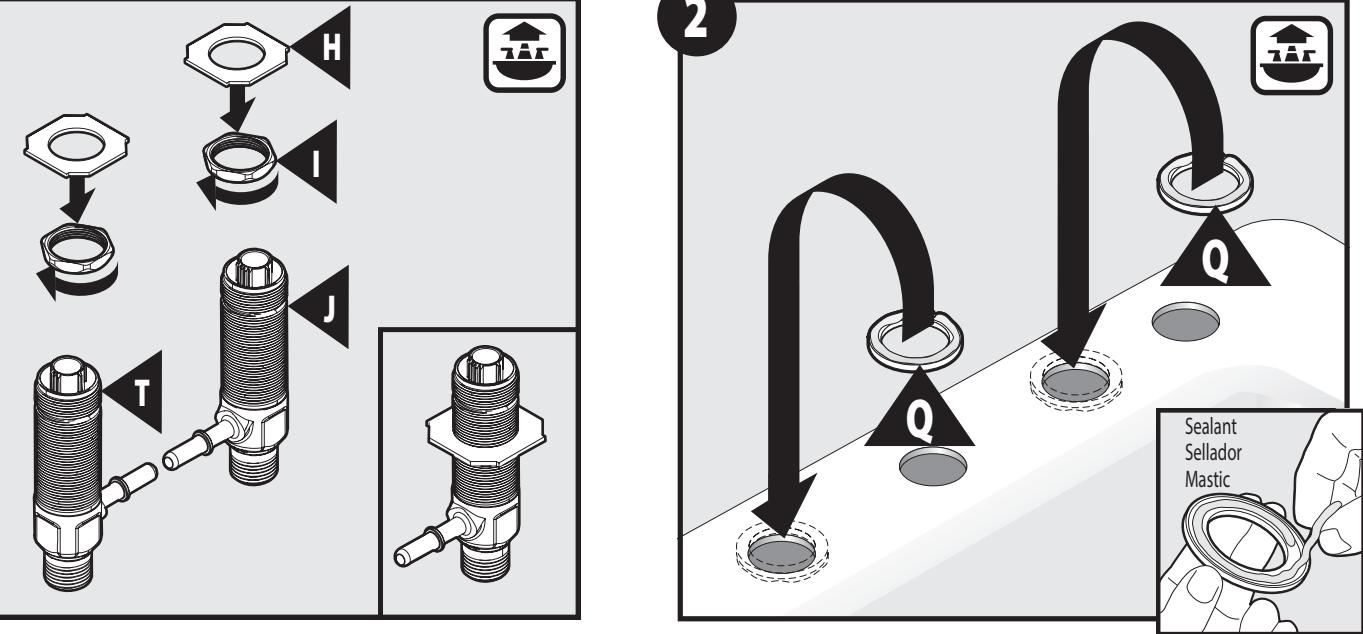
Install Lower Mounting Washers (**H**) and Valve Body Nuts (**I**) by threading onto Hot and Cold Valve Bodies (**T** and **J**).
