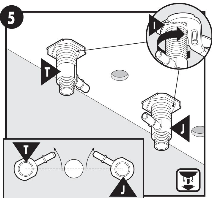
Using channel locks or a wrench, secure each Valve Body Nut (I). Point Valve Body stems out slightly to assist with Quick Connect Hose installation.
