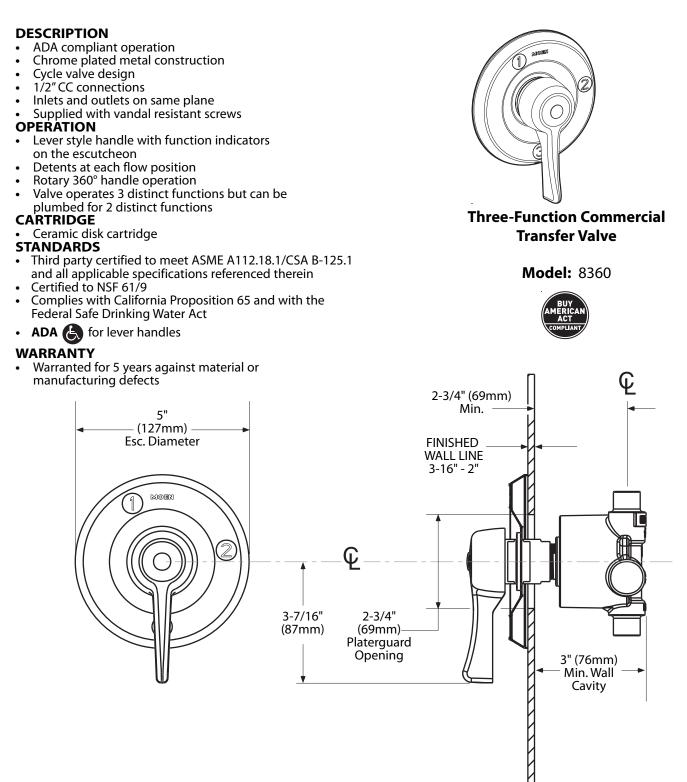
NOTE: This valve is not intended to be used as a shut-off valve. To prevent the potential of cross flow, check valves must be integral to the supply valve or installed in both hot and cold water supply lines.
