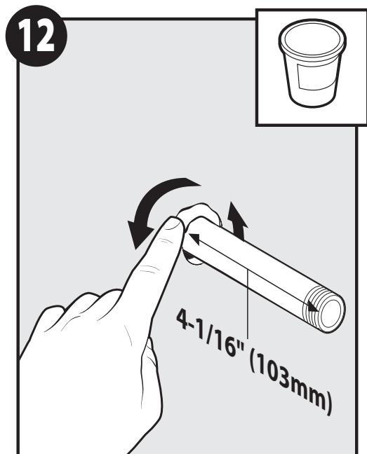
Rotate diverter knob clockwise until it stops. Insert diverter arrow (L) pointing down as shown.
