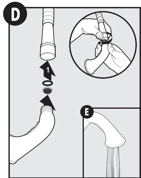
Reinstall Screen & O-Ring as shown. Thread Pullout Hose and Spray Wand. Check water flow.
