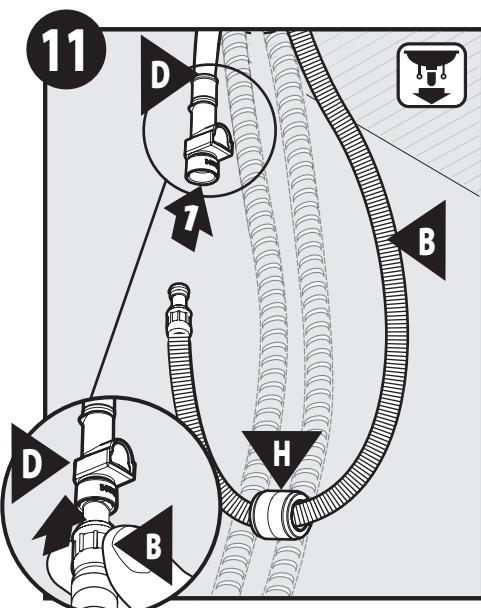
Insert Pullout Hose (B) into Duralock Quick Connect Adapter (D). Push until a "click" is heard. Tug downward on hose to test engagement.
