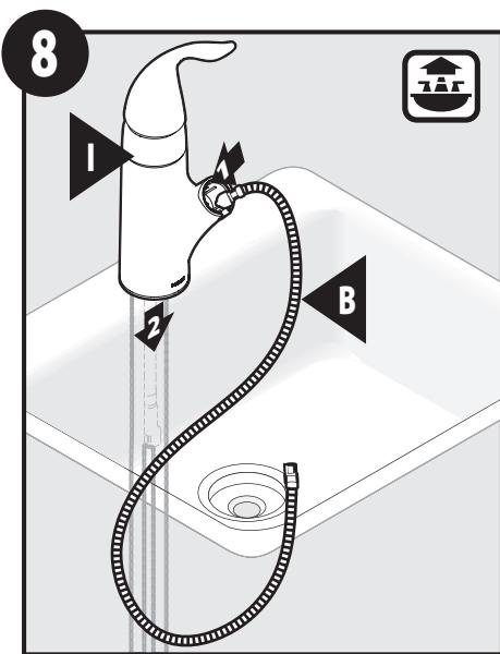
Insert Pullout Hose (B) into opening and feed through
