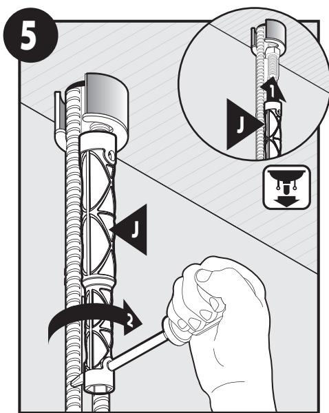
Tighten Mounting Nut with Installation Tool (J).
