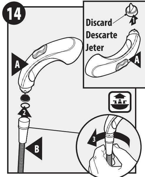
Remove and discard protective cap from Spray Wand (A). Attach Spray Wand (A) to Pullout Hose (B). Finger Tighten.
