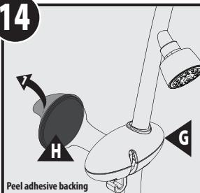
Peel adhesive backing from other side of (H). Stick mounting pad and suction cup (G) to shower wall.
