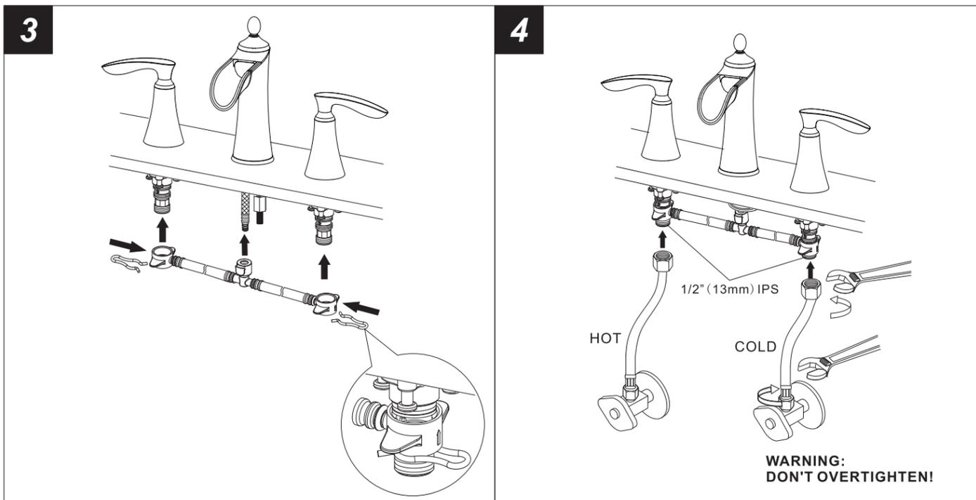
3. Position the flexible hose as shown and fix it to the faucet as shown with clamp spring.
