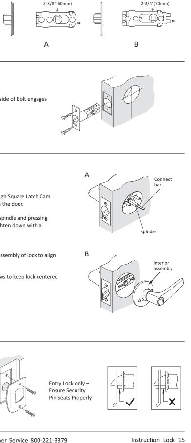
Adjust the Backset to match your door: A) To Adjust to 2-3/4" Backset pull square latch cam out.
