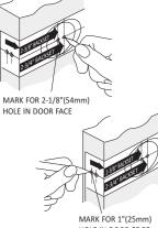
Fold Template below on Fold Line and Mark Door for Lock Bore Hole at 2-3/4" or 2-3/8" Backset and lock Edge Hole Centered on the door edge. Note: Most exterior doors
