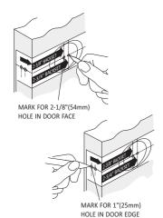
Fold Template below on Fold Line and Mark Door for Lock Bore Hole at 2-3/4" or 2-3/8" Backset and lock Edge Hole Centered on the door edge.
