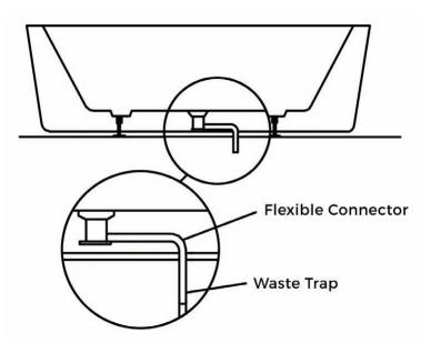
\*Flexible connector and waste trap are not supplied and must be purchased separately.
