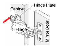
1. Unplug the cable from the Mirror Door(s) to electrical enclosure. Remove the Mirror Door(s) by pushing on the tab behind the Hinge to detach the hinge from the Hinge Plate.
