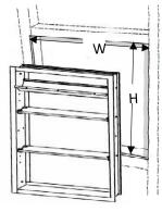
4. Frame out the wall cavity so the cabinet fits tightly into the recess.
