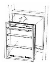
6. Insert and secure the cabinet to the recess with provided screws.
