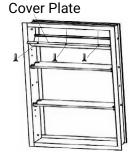
2. Loosen the electrical enclosure Cover Plate by removing the 3 screws and pivot down the Cover Plate.
