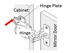
1. Unplug the cable from the Mirror Door to electrical enclosure. Remove the Mirror Door by pushing on the tab behind the Hinge to detach the hinge from the Hinge Plate.
