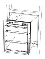
6. Insert and secure the cabinet to the recess with provided screws.
