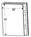
3. Measure the W (width) and the H (height) of the back of the cabinet
