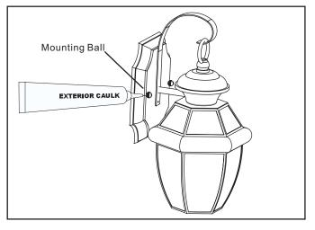
The MOUNTING BALLS require a small amount of silicone sealer to the threaded side, and then re-attach to the MOUNTING SCREWS.
