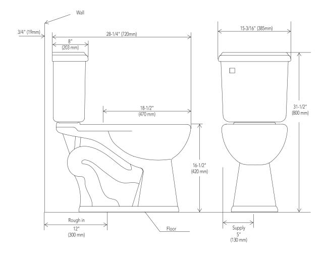
Note: All dimensions and specifications are nominal and may vary: Dimensions of 8" and greater have a tolerances of +3%. Dimensions less than 8" have a tolerances of +5%.
