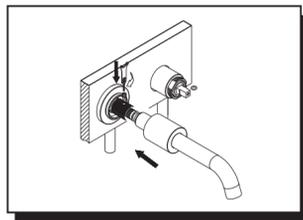
6. Install spout to spout shank: A. Slide back spout body from spout end. B. Slide spout onto spout mounting shank. Tighten set screw with hex wrench. C. Slide spout body to spout trim ring.
