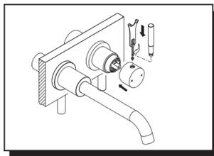
8. Install handle assembly onto valves: A. Insert handle through top of handle body. B. Slide handle assembly onto valve extension. Orient handle as desired. Tighten set screw on handle shank to valve extension.
