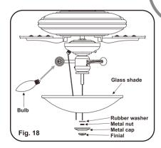
Remarked: the fan is provided extra cap and finial, which can be used when the fan is installed with univeral remote control(Not Provided)
