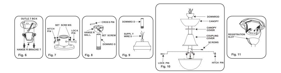
Follow the steps below to connect the fan to your house supply wires. Use the wire nuts supplied with your fan. Secure the wire nuts by wrapping the connection with electrical tape.
