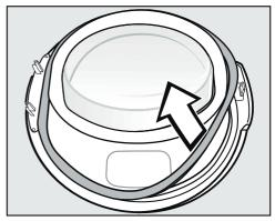
■ First take the rubber seal off the door and place this to one side.
