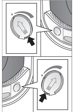
■ To open the cover, push the tab all the way up to the top.
