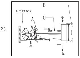
Step. 2: Connect safety lanyard(B) to Mounting Bracket(A). Attach back plate to mounting bracket and tighten ball nuts so fixture meets wall. Install fixture to back plate using two screws on side.
