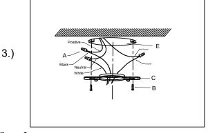
Step 3. Connect black fixture wire to positive, white fixture wire to neutral, and bare copper wire to ground using wire nuts provided.
