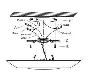
Mounting: These fixtures mount directly to most standard metallic & non-metallic electrical boxes with 2-3/4" to 3-1/2" hole spacing that are at least 1-1/2" deep. This includes 3-1/2" & 4" octagon boxes, round mud-rings for octagon and square boxes, and 3" & 4"non-metallic round boxes. Products are suitable for mounting on ceilings or walls, and are acceptable for use within closet storage spaces when installed per NEC requirements.
