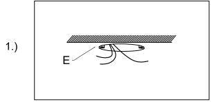
Step 1. Bring positive, neutral, and ground supply conductors (120V, 60Hz) to the room side from junction box(E).
