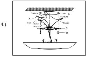
$Step\ 4.\ \ \mbox{Align fixture spring with cutout in mounting strap} \ \mbox{and press towards mounting surface to snap into place}\ .$
