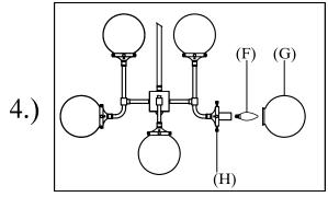
step4: Loosen the lock screws (H). Install E12 bulb(F) and attach glass (G). Secure glass (G) by tightening lock screws (H).
