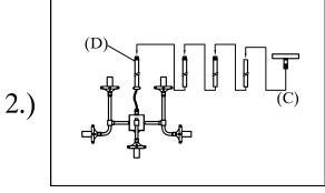
step2: Carefully remove packaging from fixture. Run wire through stems (D) and combine stem lengths to meet desired mounting height. Then attach canopy (C) to fixture.
