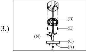
step3: Wire fixture to wires in outlet box. Copper wire in canopy is for grounding. Install canopy (C) to mounting bracket(B) using ball nuts (A) to secure.
