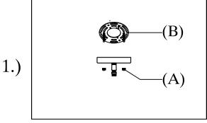
step1: Remove mounting bracket (B) from fixture and install to electrical box
