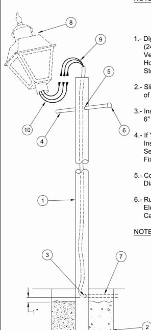
NOTE: It is recommended that the section of Post Bottom to be placed in the Concrete, be coated with an Asphalt Paint containing Aluminum Pigment. This is Especially Important in areas where the Soil is high in Acid or Alkali content.
