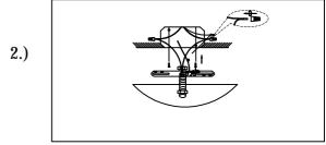
Step.2: Wire fixture to wires in outlet box. Copper wire is for Ground.
