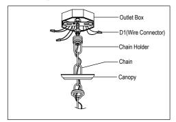
3. Wire fixture wire leads to outlet box wires. Wire copper ground wire from fixture to ground from outlet box. Pull canopy and screw ring up chain to ceiling and tighten securely.
