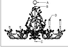
1.Install top loop A to center stem and attach appropriate amount of chain to loop to achieve desired mounting height. Thread wire through every 3rd loop of chain.
