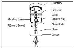
2. Remove ring from loop and slide down chain.
