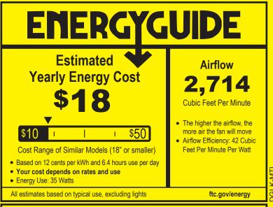
Airflow Shown Is a Weighted Average of High and Low Cubic Feet per Minute Based on Downrod
