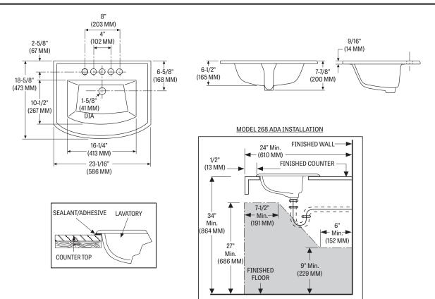
Fixture performance and specifications meet or exceed ASME A112.19.2-2013/CSA B45.1-13 standards, and other state and local codes.
