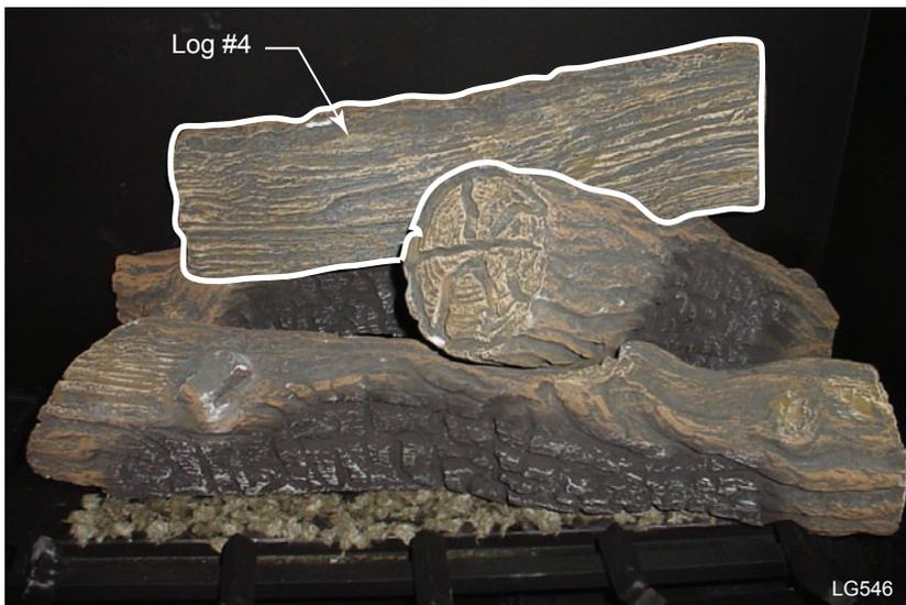
5. Place log #4 by matching the rectangular protrusion on the bottom of this log over the rectangular notch on log #1, then swing the log slightly toward the front and set the log over the notch located on the upper surface of log #3. *Figure 68*
