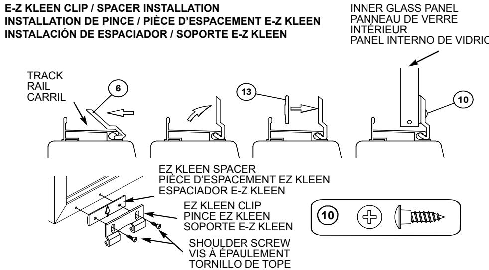
**Please note**, when installing the Shoulder Screws, **DO NOT** use a power screwdriver, use a #2 phillips head screw driver, **DO NOT OVER TIGHTEN**.
