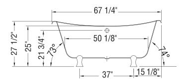
Bathtub base includes anti-vibration Neutra-Phone leg supports (not shown). All dimensions are approximate. Structure measurements must be verified against the unit to ensure proper fit.
