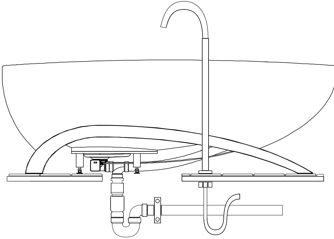
Install the access panels on both sides of the bathtub and assemble them with the magnets (Fig.11). Then lift the access panels and insert the spacer to secure them in place.
