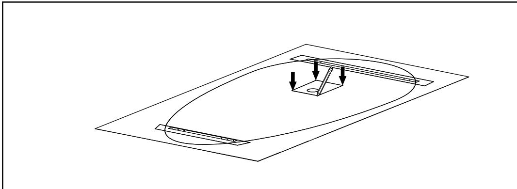
Remove the template and cut an opening in the floor along the lines of the shape formed by these four marks.
