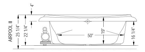
Pump is at 9 o'clock when drain is at 12 o'clock.
