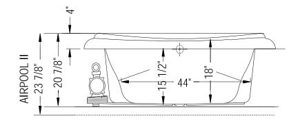
Pump is at 9 o'clock when drain is at 12 o'clock.
