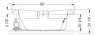
Pump is at 9 o'clock when drain is at 12 o'clock. Bathtub base includes non-adjustable Neutra-Phone leg supports (not shown). All dimensions are approximate and subject to change without any prior notice.
