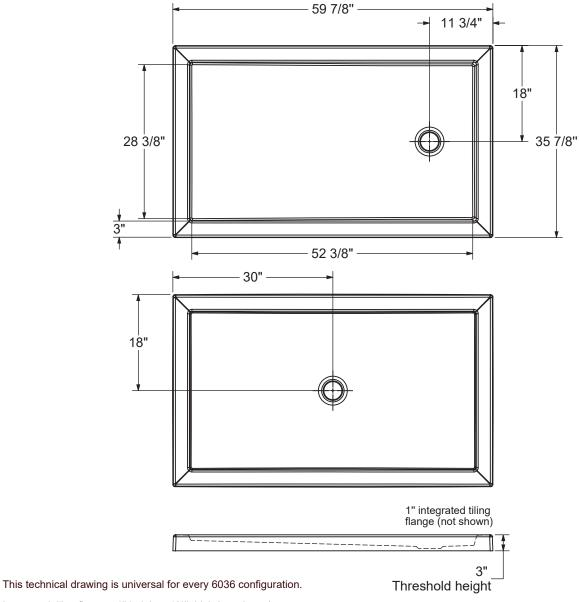
Integrated tiling flange : 1" height x 1/4" thick (not shown) Tiling flange position is determined by chosen configuration.
