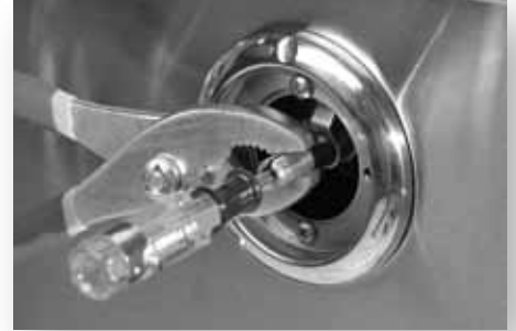
Use a small screwdriver for low setting burner adjustment.
