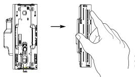
Grasp front module on sides and pull to remove.
