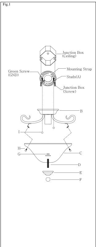
MIN 90°C SUPPLY CONDUCTORS
