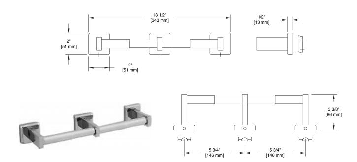
MATERIALS: Inner Wall Flange - 16 gauge type 304 stainless steel
