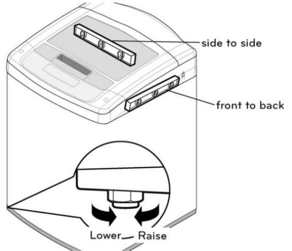
If the washer is not level, adjust the leveling feet. Turn clockwise to raise, counterclockwise to lower.
