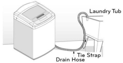
Bend the end of the drain hose to the desired shape and support it on the edge of the laundry tub. Use a tie strap to secure the drain hose in place.
