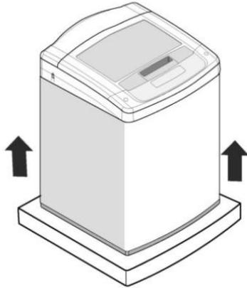
When removing the washer from the carton base, be sure to remove the tub support in the middle of the carton base. If you must lay the washer down to remove the base packaging materials, always protect the side of the washer and lay it carefully on its side. Do NOT lay the washer on its front or back.
