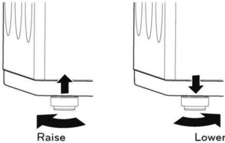
3 To make sure that the washer is properly level, open the lid and look from above to see if it is same as shown below. If you have a level, check your washer with the level.
