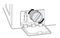
**8** Close the drain pump filter cover.
