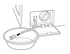
**4** Remove the pump filter.
