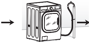
Connecting the drain line
