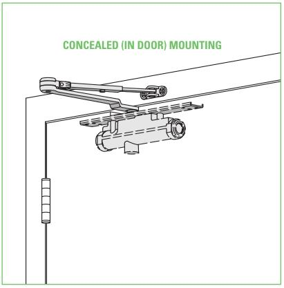
The concealed 3030 is designed to mount in a 1 3/4" interior door. The double lever arm provides superior door control and the choice of finishes and arm functions meet virtually all architectural requirements.
