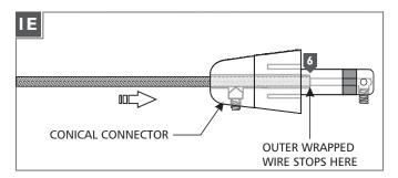
6 Feed and push the coaxial cable into the conical connector. The coaxial cable will come to a stop point after being inserted 3/4" into the conical connector.
