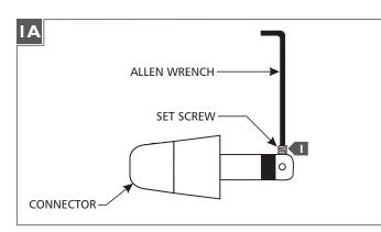
Back out (do not remove) the set screw on tip of the connector with the provided Allen wrench.
